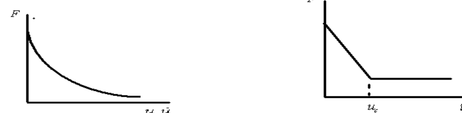
Figure 2. Left panel shows hyperbolic friction laws that weaken hyperbolically with slip or slip velocity. These laws have no inherent scale. The right panel shows the traditional slip weakening friction that has an inherent length scale u_0 .
